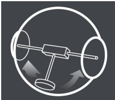
Fig.9: A commercialized pendulum-driven robot. Rotundus [3].
